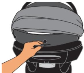
both L.S.P, then lift seat cover over L.S.P. locks and away from back of seat.
