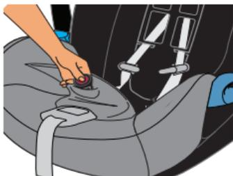
3. Replace the backrest cover, being sure to pull it over the tabs on the inside of the seat shell.
