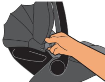
9. Replace the Headrest Cover. Snap the two snaps to attach it to the Harness, then snap the two snaps behind the headrest.
