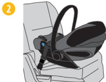
If necessary, tuck the loose end of the **LAP BELT** out of the way.
