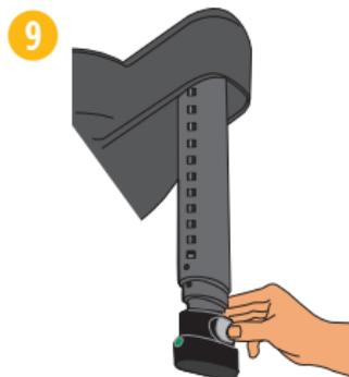
Use the **FIRST** hole that will lock the Load Leg Foot firmly against vehicle floor.
