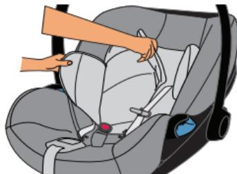
4. Pull Headrest Cover forward. Unsnap the two snaps behind the headrest, then unsnap the two snaps to separate it from the Harness.
