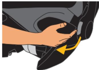
**To Retract the L.S.P. Device**, depress the button, push the L.S.P. Device back into the carrier, and listen for an audible **CLICK**.
