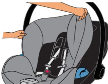
4. Extend the L.S.P. Device on both sides of the seat.
