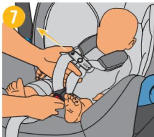
8. Slowly pull the Adjuster Strap to tighten the Shoulder Straps. A snug strap should not allow any slack. It lies in a relatively straight line without sagging. It does not press on the child's flesh or push the child's body into an unnatural position.
